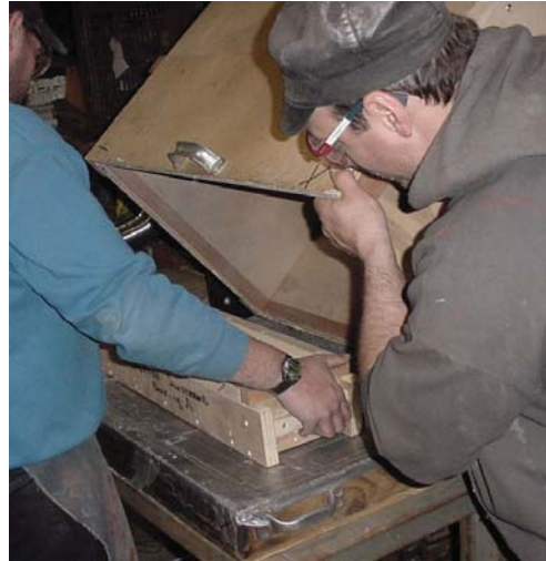
Figure 2-1 Custom Mold Curing Emissions Enclosure
