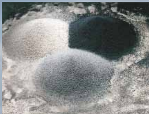
Thermally reclaimed sand (bottom), is shown with new sand (left) and spent sand (right).
