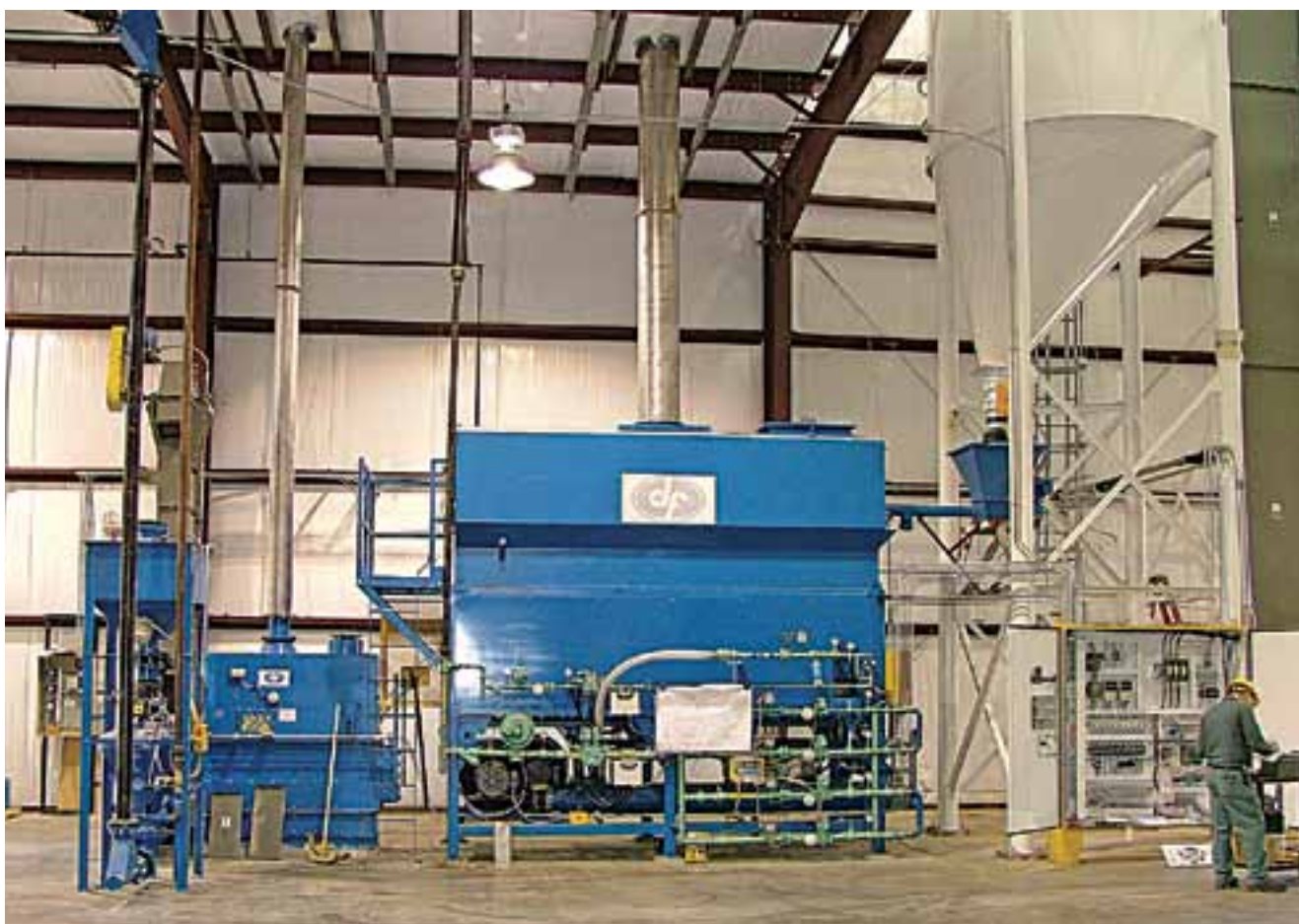
Thermal sand reclamation systems (two examples are pictured above and below) heat sand additives to combustion and separate the ash and sand fines from reusable sand particles.
