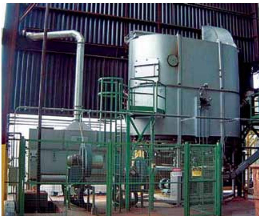
Thermal sand reclamation systems (two examples are pictured above and below) heat sand additives to combustion and separate the ash and sand fines from reusable sand particles.
