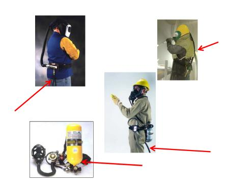
A source of **breathable** air is supplied to the facepiece. Only air supplied styles can be used in IDLH environments.
