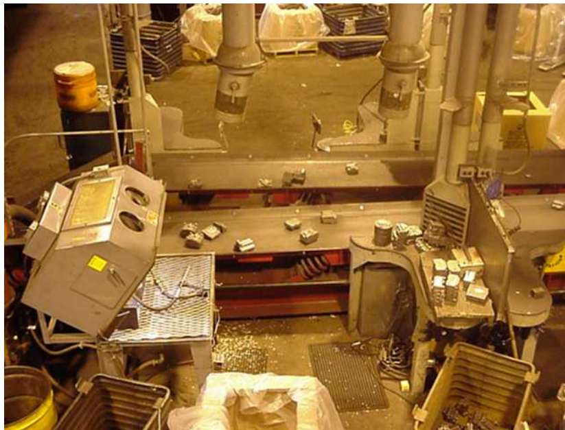
Figure C-4. An inspection station equipped with an exhaust hood and air drops.
