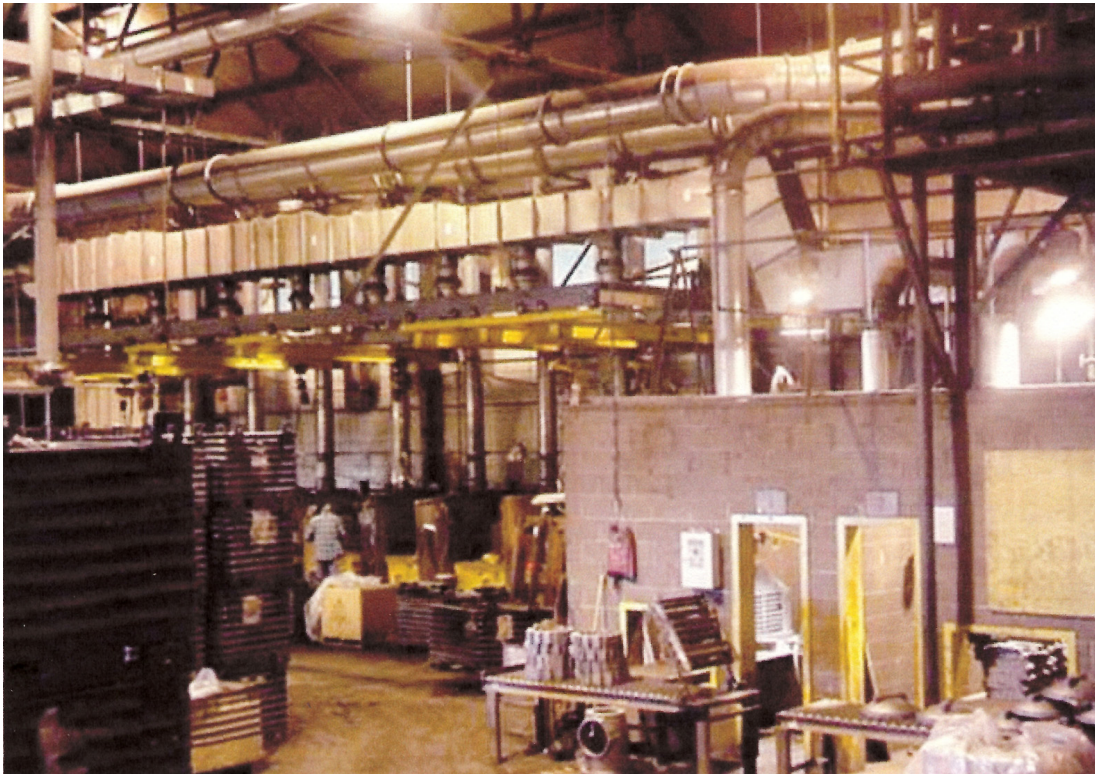
Figure C-1. Large casting grinding is done on ventilated workbenches in semi-enclosed booths (center) and in enclosed booths (right).
