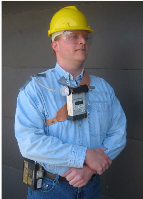
Figure 3-1 Worker wearing portable real-time monitor for respirable dust.
