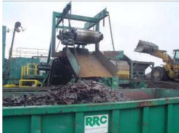
Photo 2: Metal being recycled out of the foundry sand.
