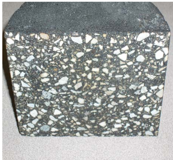
Photo 1: A core taken from a test pad at the construction site.
