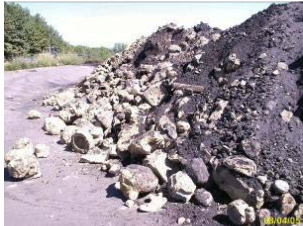
Photo 2: Some of the fragments that did not break up as expected.
