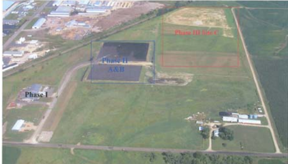
Photo 2: An aerial view of the industrial park under development. Phase 1 is furthest left in the bottom corner of the picture and already occupied by buildings. Phase 2 is in the center, faintly outlined in blue. It has been temporarily capped with asphalt. Phase 3 is furthest right, faintly outlined in red. It has been restored with topsoil and seeded.
