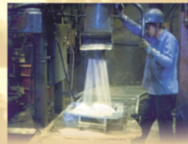
Mid-City Foundry of Wisconsin processes up to 36 tons of sand daily, reusing it up to 20 times, compared to the industry average of eight, before disposal.
