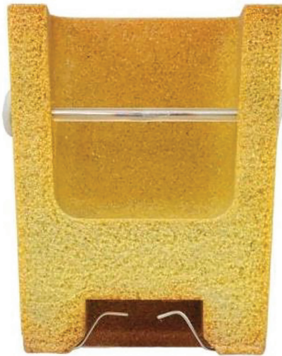
a) sand cup with disposable thermocouple
