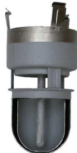
b) steel cup (SinterCast) with two thermocouples in the protective tube
