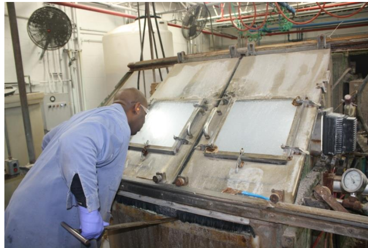
Removing Ceramic with Water Blast
