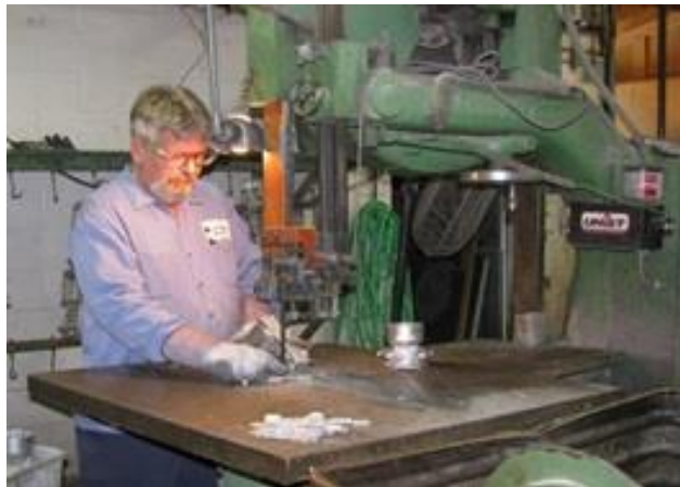
Cut-off operation with band saw
