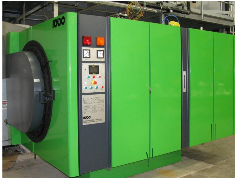
Steam Boilerclave to de-wax shell
