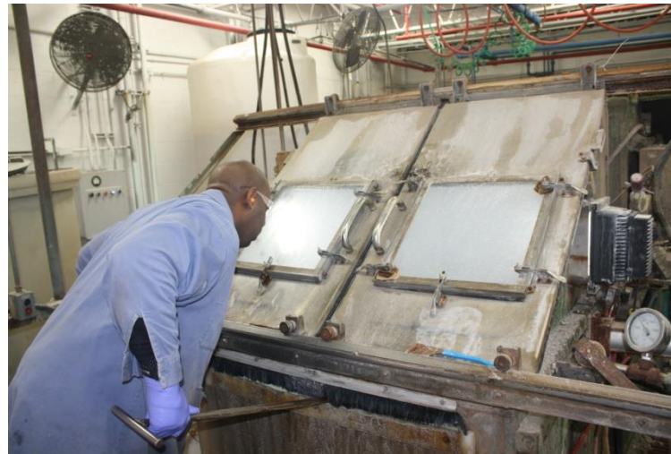
Removing Ceramic with Water Blast
