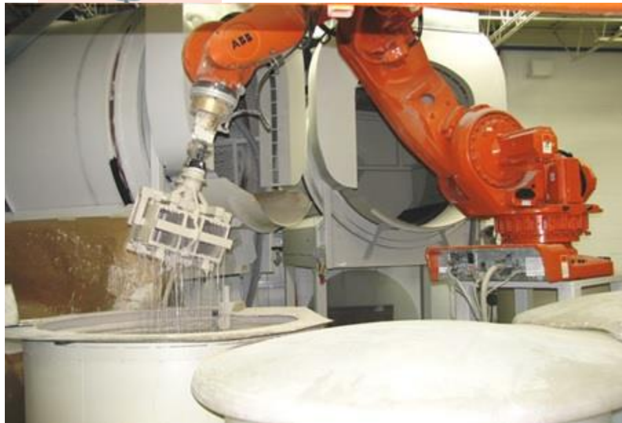
Layer of Ceramic Shell being applied by robot
