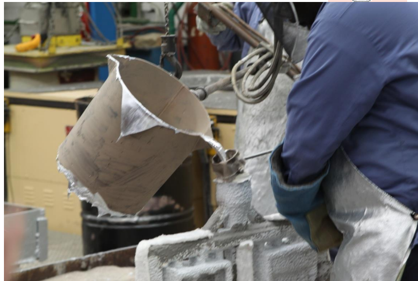
Casting Ceramic Shell with Ladle
