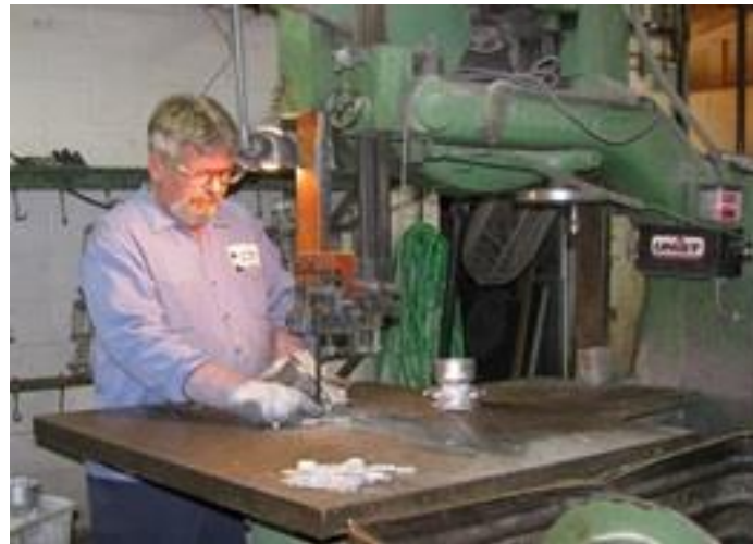
Cut-off operation with band saw
