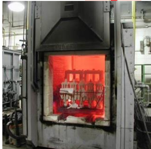
Ceramic Shells being Fired
