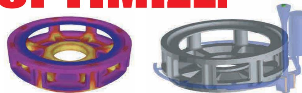
**From Unrigged Casting to Fully Rigged Model**
